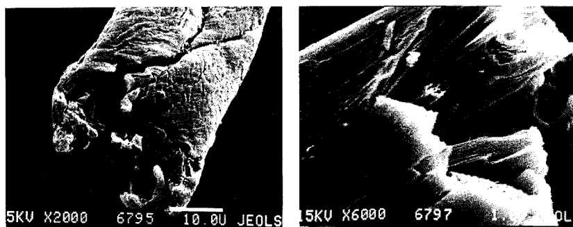
Fig. 5 (A-D). SEM micrographs of the initial MCC fibre (A) and the complexes MCC-trypsin (B, C - after trypsin adsorption to MCC; D - after trypsin desorption from the complexes)
